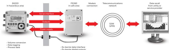
The Ex-barrier of the serial interface and the pulse outputs of the volume converter is provided by function extension unit FE260. In addition, the intrinsically safe power supply
