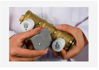
Remove the manual handwheel with a screwdriver and place the thermo-electric actuator on the valve, turning it about 15° until a click click of engagement is heard.
