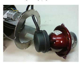
4b-2: Position lamp removal tool over locking ring as shown below. Twist approx. 30 degrees anti-clockwise.
