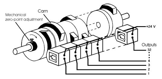
Picture 1: Mechanical cam control
