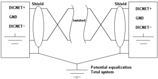
The minimum wiring with shielding between two bus users is shown in the following illustration:
