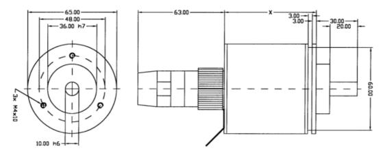
Picture 2: Dimensional drawing ROTARNOCK RS232 or RS485, option IF, version IP65
