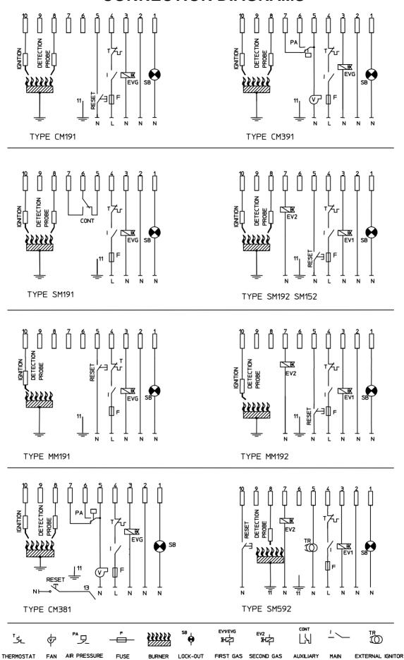
**NOTE:** the limit thermostat has to be wired in series to the live.
