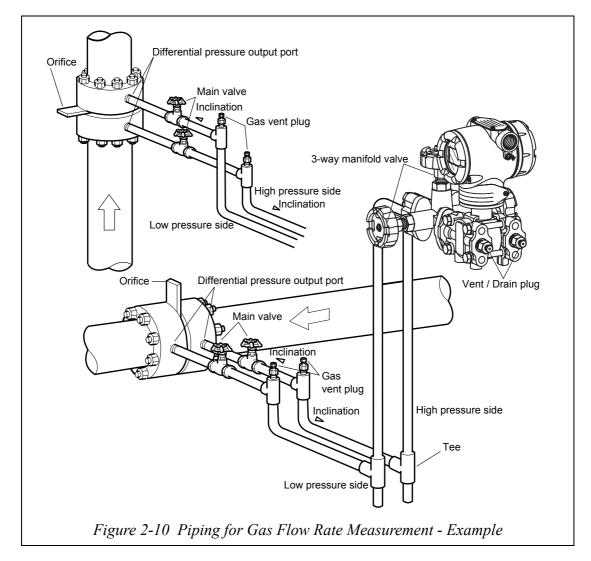
This transmitter is located above the differential pressure output port of the process pipe.
