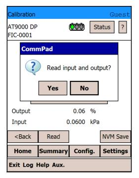
(4) Input has now changed approximately to zero as a result of the calibration.
