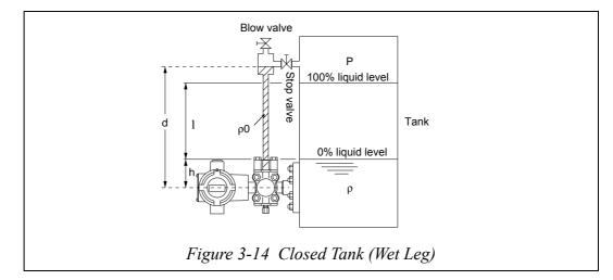
Differential pressure at 0% liquid level (Pressure on high-pressure side - Pressure on low-pressure side) =  $d\rho_0 - h\rho = LRV$
