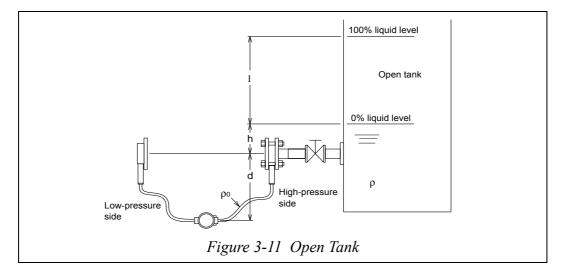
Differential pressure at 0% liquid level (Pressure on high-pressure side - Pressure on low-pressure side) = hr = LRV
