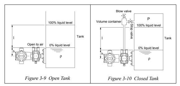
Differential pressure at 0% liquid level (Pressure on high-pressure side - Pressure on low-pressure side) =  $h\rho$  = LRV
