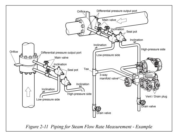
This transmitter is located under the differential pressure output port of the process pipe.
