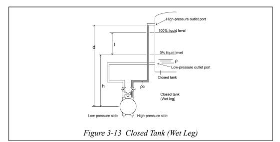
Differential pressure at 0% liquid level (Pressure on high-pressure side - Pressure on low-pressure side) =  $d\rho_0 - hr = LRV$
