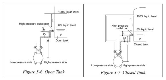
Differential pressure at 0% liquid level (Pressure on high-pressure side - Pressure on low-pressure side) =  $h\rho + d\rho_0 = LRV$
