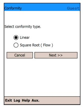
(3) If you select square root conformity, a screen for selection of low flow cutoff appears. Select either "default 7.1%" or "Custom value(0- 20%)" which allows the choice of any value between 0% and 20%.
