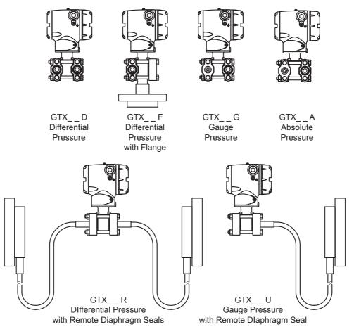
Figure 1-1 AT9000 Advanced Transmitter Family
