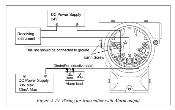
~Note Current cannot checked for a transmitter with alarm contact output.
