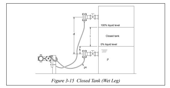
Differential pressure at 0% liquid level (Pressure on high-pressure side - Pressure on low-pressure side) =  $d\rho_0 - h\rho = LRV$
